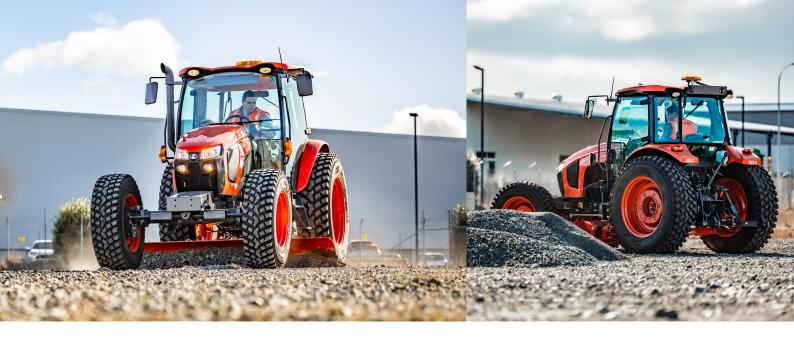
**STANDARD w OPTIONAL BROOM** 5,070kg 5,370kg **WEIGHT LENGTH** 4,420mm 5,800mm 2,210mm 2,210mm **TRACTOR WIDTH** 2,800mm 2,800mm **SLEWED WIDTH** 3,050 mm (10ft) 3,050mm (10ft) **GRADER BLADE WIDTH** 22.5° each way **SLEW ANGLE** 22.5° each way 185mm 185mm **BLADE CLEARANCE** (FULLY RAISED)
